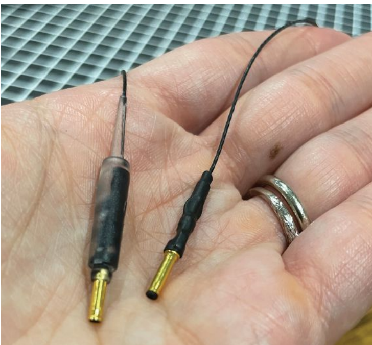
▲ The finished connector on the left is seen here with transparent overmolding. The overmolding process includes a polymer 3D printed piece seen at the top.
