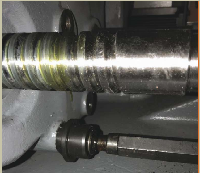
The ejector plate here is nearly coupled. As the barb is inserted into the coupler, it will reach a point where the collar on the outside of the coupler will click forward, creating a solid connection.
