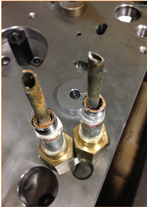
This partially blocked bubbler was removed from a mold due to its degraded performance.
