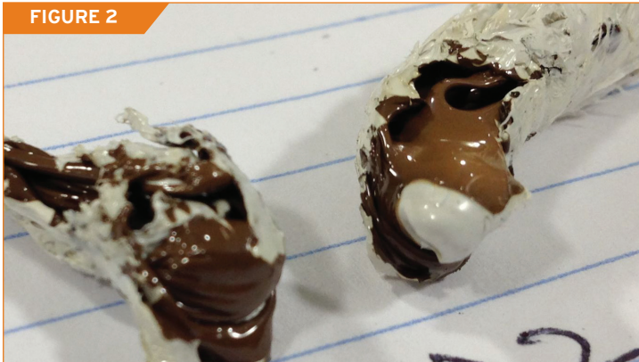
This example of skinning is marked by the degraded "brown" material forming a skin. The plastic was pulled out of a hot runner manifold's inlet immediately after the screw.
