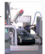
Sprue remover Cod. RB020PM Pneumatic with belt for removing sprues. 230V 50Hz
