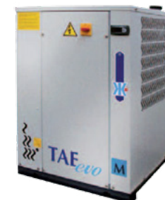
Chiller Cod. RB002M10 Chiller - Pot. Cooling power 4,4 Kw – Power rating 1,4Kw - 593x575 h.785 - peso 60 Kg - 230V/1/50Hz
