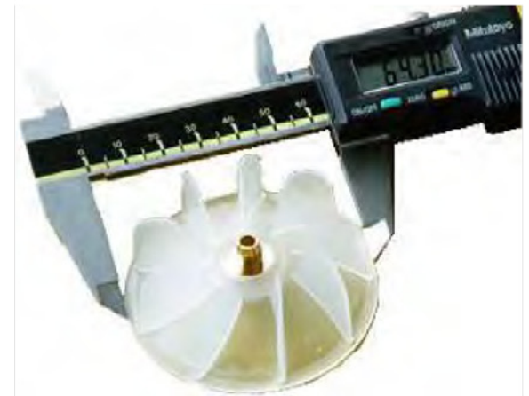
PP - 1 cavity - insert loaded by robot
