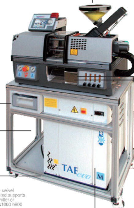
Mould cabinet Cod. RB008CS Mould cabinet (can hold up to 12 moulds.) rotating shelves - 600x520mm
