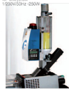
De-humidifier Art RB002DE Capacity 2 l. - max temp. 180°C Complete with venturi loader and adapter for Babyplast 1/230V/50Hz -250W
